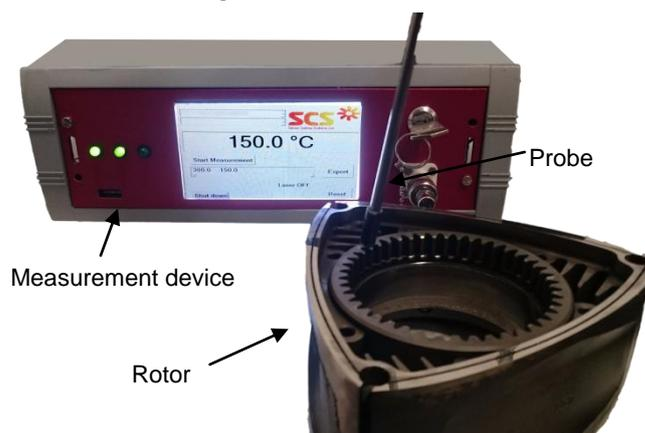
*A measurement in action on the rotor*
