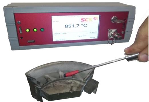
Figure 1. A measurement in action on the NGVS.
