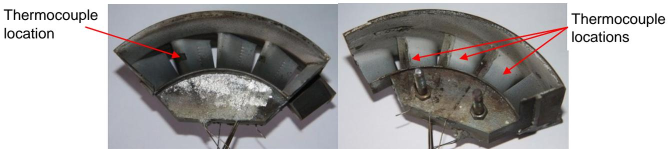
Figure 2. A photograph of the (left) front and (right) back of the NGVS after operation.
