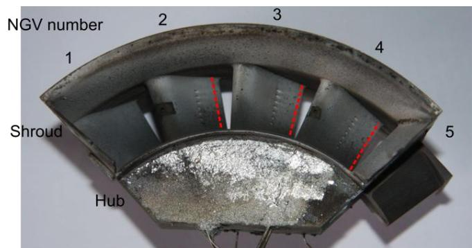
Figure 3. A photograph of the NGVS showing the locations of the measurements using THP on the trailing edges as red dashed lines.
