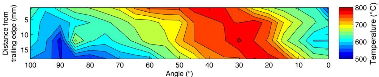
Figure 7. The temperature measurement results on the shroud surface shown in Fig. 5 represented as a contour plot. The contours are at every 20°C.
