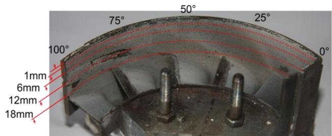
Figure 5. A photograph of the shroud with the four measurement lines labelled.
