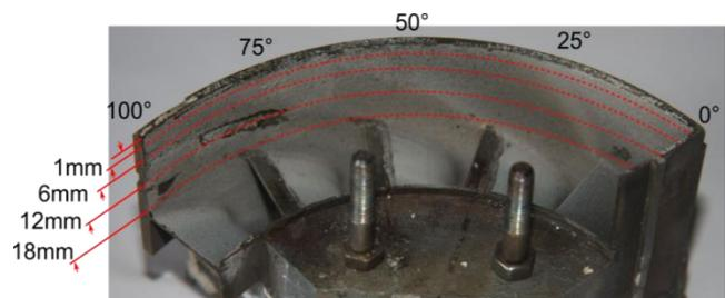
Figure 5. A photograph of the shroud with the measurement lines labelled.
