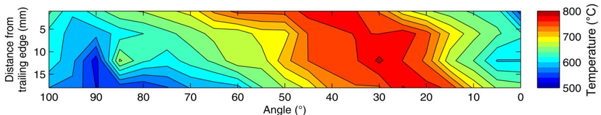
Figure 7. The temperature measurement results on the shroud surface shown in Figure 5 represented as a contour plot. The contours are at every 20°C.
